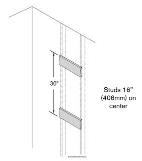
Fig. 22 Distance between support boards
